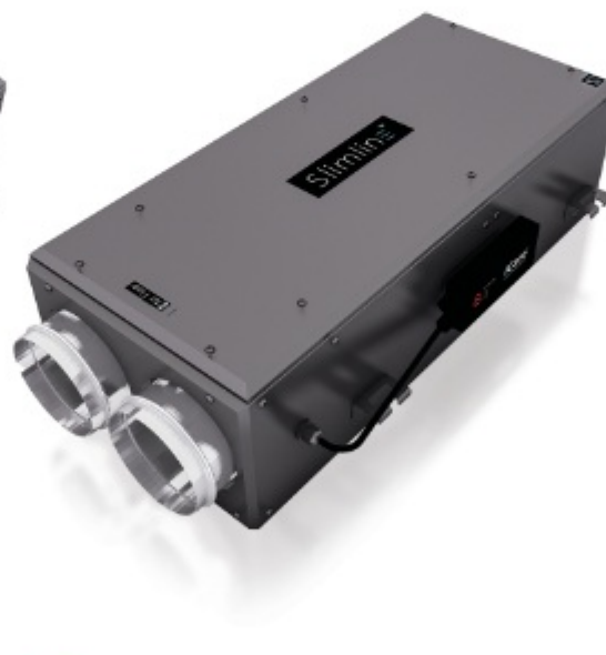
2 | Slimline S2 2-Stage Filtration Unit (Coarse Dust/Activated Carbon - HEPA) Ceiling-mount (Recessed/Exposed) Backward-Curved Centrifugal Fan
